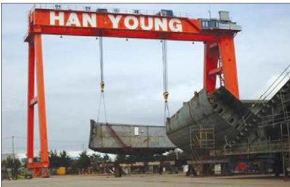
▶ Gantry crane 320tons
