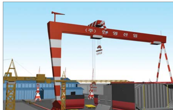
▶ 700ton goliath crane to be installed
