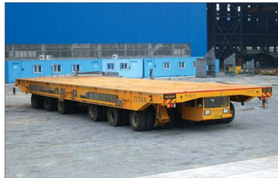
▶ 320ton transporter / 6m(W) x 18(L) _ 2 units
