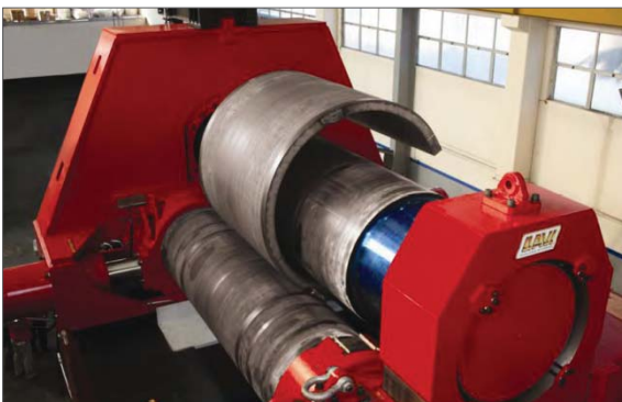
▶ PRESS-ROLL BENDING M/C 1,00MM x 3,600W
